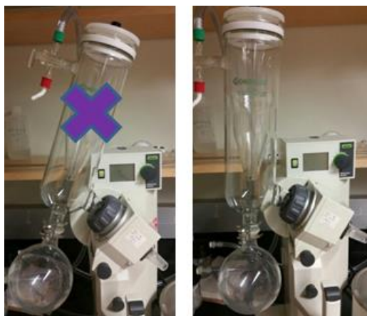
Figure 1. A condenser in a bad position (left) and a good position (right)
