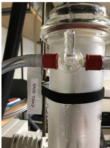
Figure 2. Valve on the condenser at the "closed" position.
